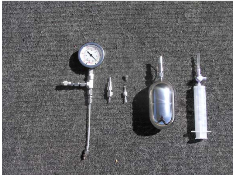
Photo 1 – Soil gas sampling materials: sample collection train, vapor implants, mini-can (400 cc), purging syringe.
