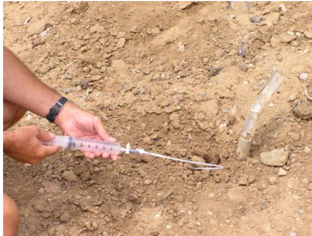
Photo 5 – Collecting sample with 60 cc syringe. Note small dead-volume of tubing connecting syringe to implant.
