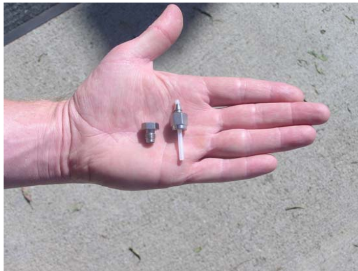
Photo 2 – Sub-slab vapor implant (1/8" OD) and cap. Nylon tubing can be cut to any length.
