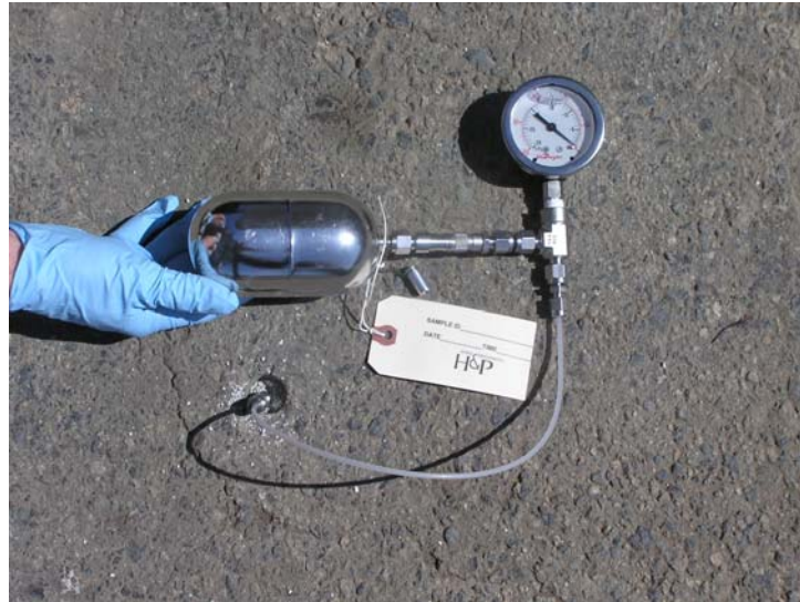
Photo 7 – Collecting soil gas sample in mini-can (400 cc).
