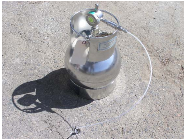
Photo 8 – Collecting sample in larger canister (6 liter). No sampling train is required since the canister is already equipped with valve, vacuum gauge, and flow choke.
