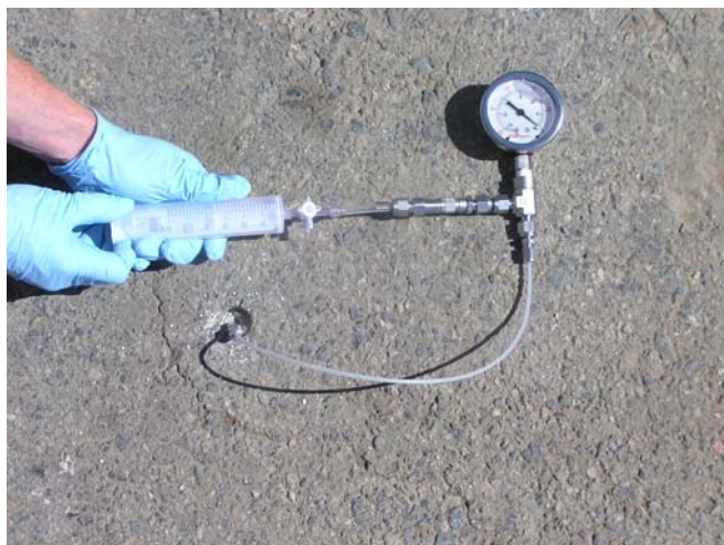
Photo 6 – Purging implant & sampling train with 60 cc syringe. Note small dead-volume of tubing connecting syringe to implant.
