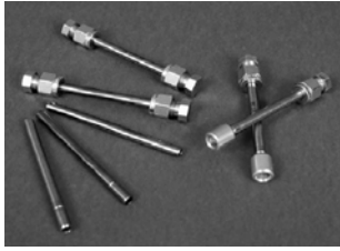
Adsorbent inside tube open on one end
