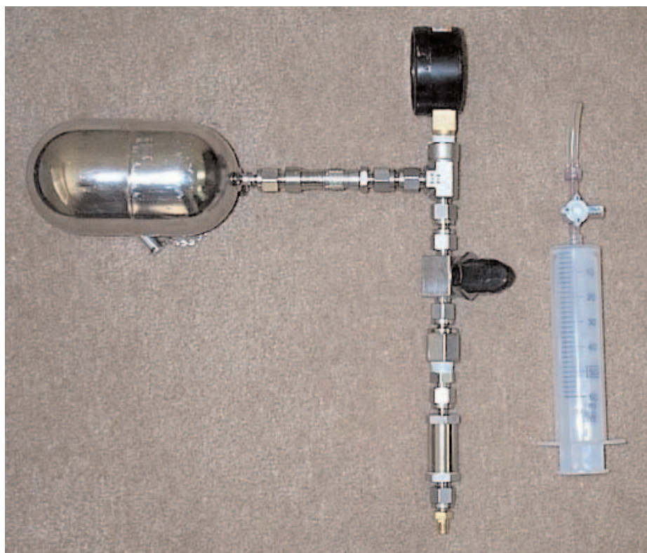
FIGURE 2. Comparison of a sampling train provided by a lab to fill canisters for off-site analysis vs. a syringe used for on-site analysis. The larger dead-volume and numerous connections of the sampling train increase the chances of equipment blanks and leaks.
