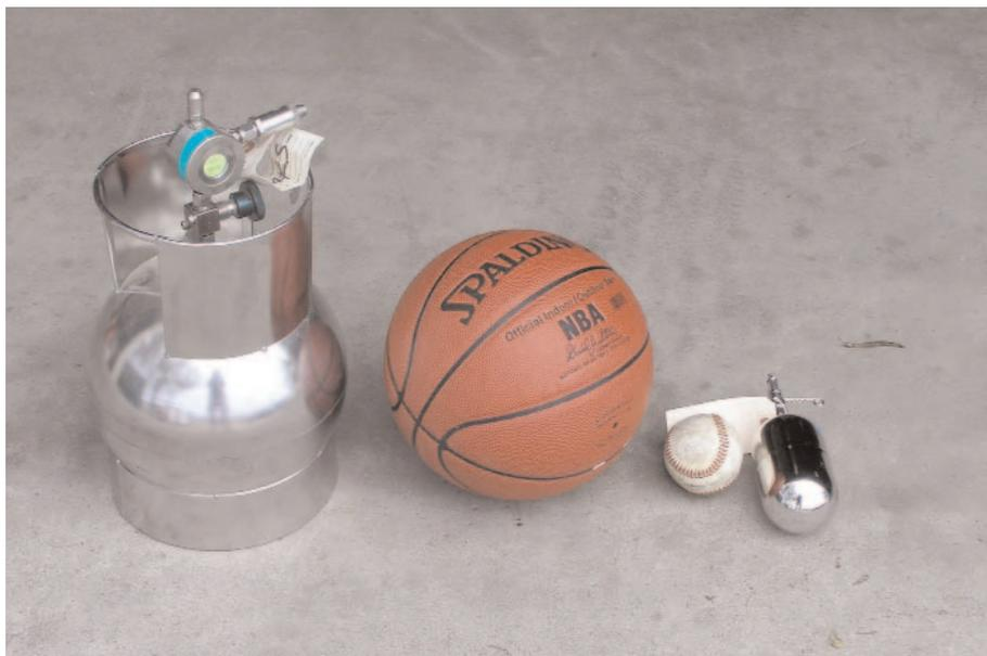
**FIGURE 1.** A basketball or a baseball? The 6L Summa canister has a volume about the size of a basketball, whereas the mini-can has an approximate volume of a baseball.
